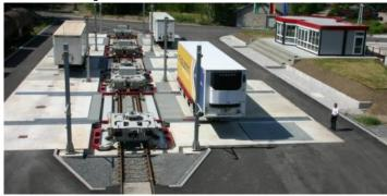
RailRunner (below) is a North American solution requiring specialised semi-trailers with reinforced frames that may be placed on bogies to be forwarded on rail without the use of wagons.
