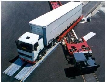
Nikrasa (to the right) is a frame and ramp system enable the vertical loading of non-craneable semitrailers onto pocket wagons compatible with the Nikrasa frame.
