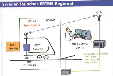
HE first pilot operation of ERTMS Regional will take place in Sweden this summer. The basic aim of the ERTMS Regional concept, pioneered by the UIC and being applied in a real application by Sweden's infrastructure manager Banverket, is to provide cost-effective solutions when renewing or introducing signalling equipment on regional and local lines.
