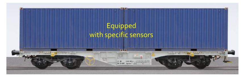
Loading unit / cargo monitoring (ILU owner & goods, RU) Predictive maintenance (wagon keeper) Load optimisation (axle weight, total weight, composition) Data transfer and sharing (RU, wagon keeper)
