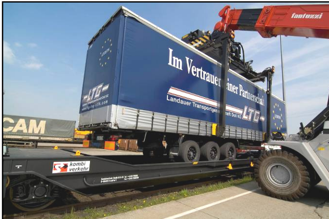
Loading of mega-semi-trailer on the new wagon
