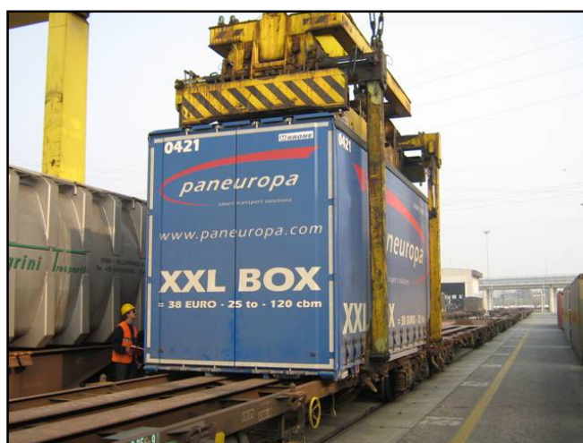
Loading of swap body on a CEMAT’s Multifret wagon
