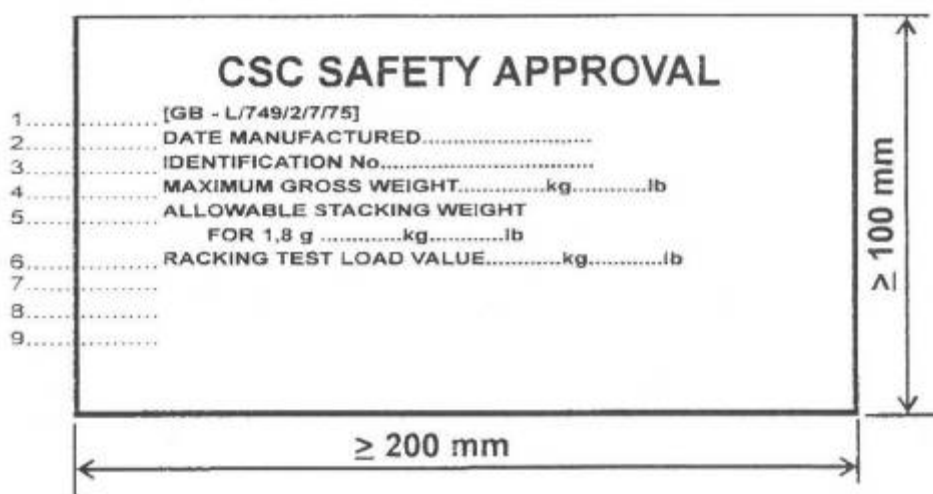
Figure 8.10.7-4: Safety approval plate on container
