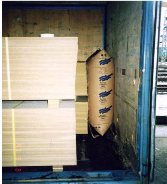
Picture 19: Air cushion in a semi trailer
