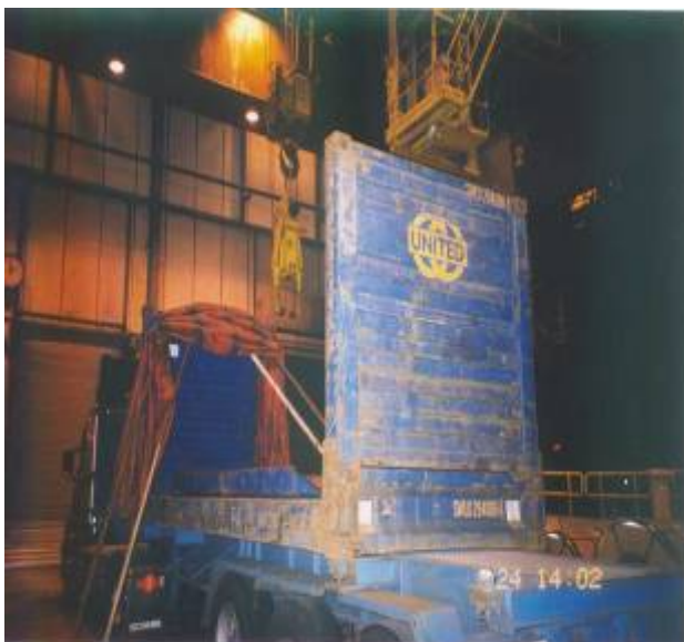
Flatrack with a cover and groove
