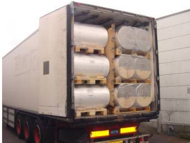
Picture 18: Filler between the rows of cargo
