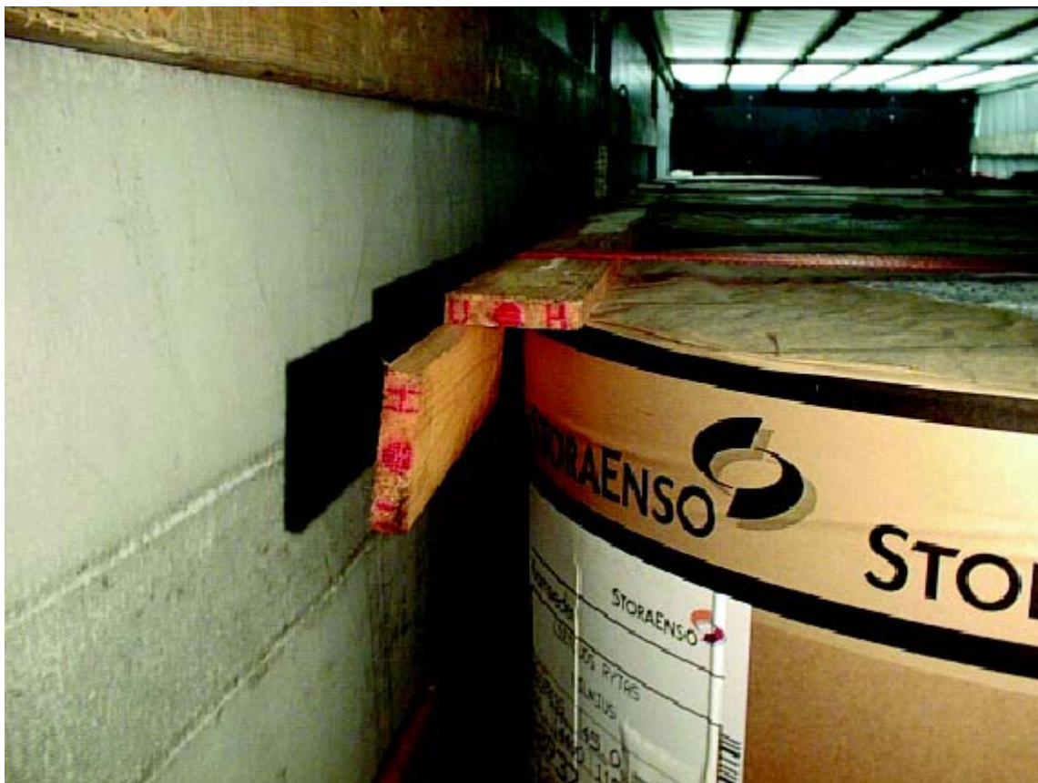
Picture 53: Edge beam made of wooden boards.
