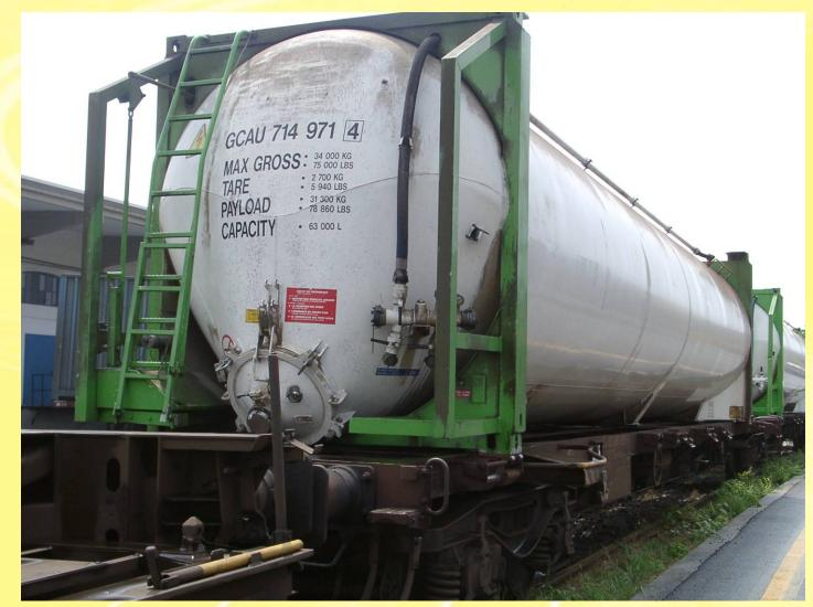
This type of tank SB with top corner fittings is longer and wider than 40' ISO tank containers
