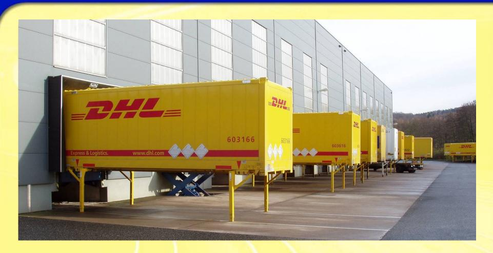
The legs allow the truck to deposit the SB at the warehouse or to transfer between trucks – no transhipment cranes are needed. A lot of SB are used in pure road traffic.
