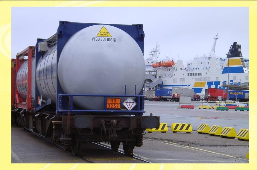
This type of tank SB with top corner fittings is longer and wider than 20' ISO tank containers.
