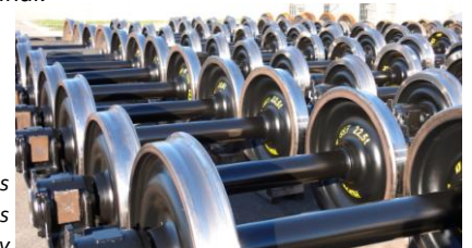
Renovated axles awaiting to be fitted onto wagons at Hupac's new maintenance facility
