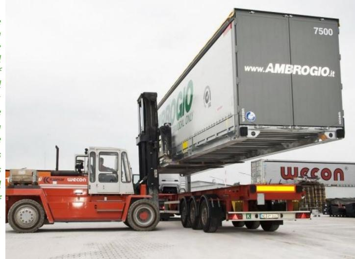
*Consequence of the* currently ongoing revision of Directive 96/53 on weights and dimensions of commercial road vehicles: 15cm extension to the semi-trailers carrying pallet-wide 45-foot containers or swap-bodies has been allowed enabling the use of rectangular 45 footers.
