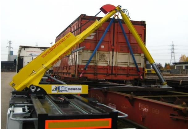
Figure 25 Sidelifter Source: http://www.boxmover.eu/spool/gfx/1321259759KL\_Container\_OEBB\_Umschlag\_\_058.jpg
