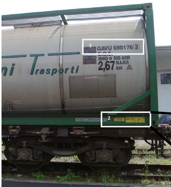
White frame 1 = BIC-Code white frame 2 = codification plate in the picture above
