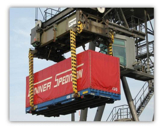
Minimum tare weight through lighter construction: 2.5t for a 7.45m and 4.9t for a 13.60m
