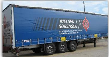
Standard semi-trailer with length of 13,60m (width of 2,55m or 2,60m – height of 4,00m )
