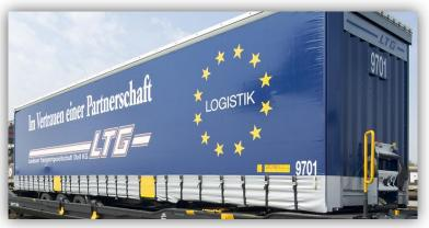
MEGA semi-trailer with length of 13,60m (height of 4,00m)
