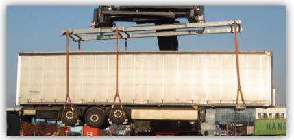
ISU technology for transporting semi-trailers up to 4 m and 2,60 m
