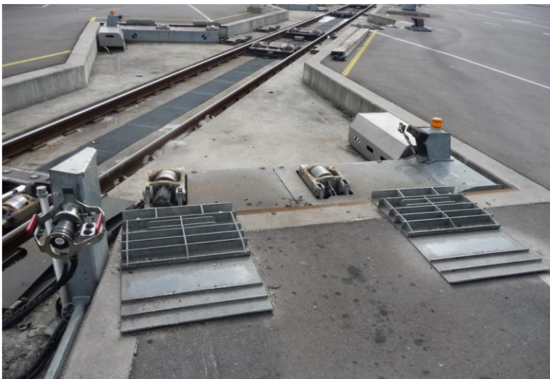
Figure 4-4: Transshipment equipment for the Modalohr horizontal technology
