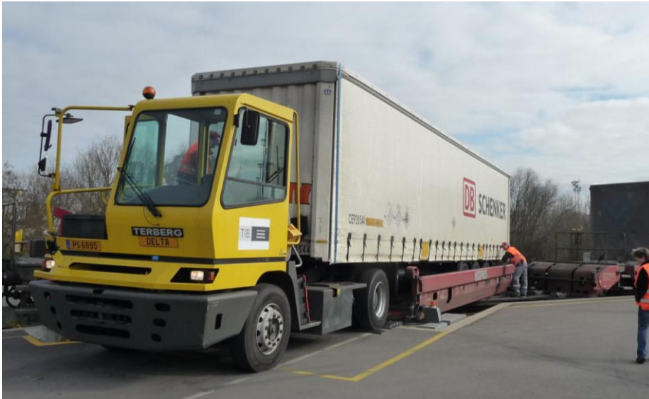
Figure 4-5: Unloading a semitrailer with the Modalohr horizontal technology
