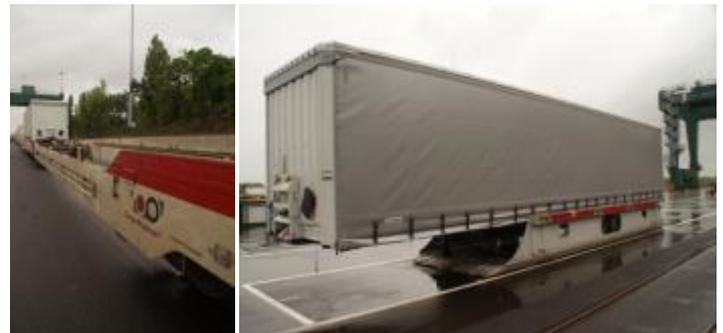
The Köln Nord Terminal was established to accommodate the technological requirements of CargoBeamer, a technique which combines a steel tray and a specially configured wagon to enable the vertical transshipment of non-craneable semi-trailers (see pictures above) - opening a new possibility for these ordinary semi-trailers to be forwarded by unaccompanied CT as well. More information about the CargoBeamer technique can be found here: <http://www.cargobeamer.eu/#>
