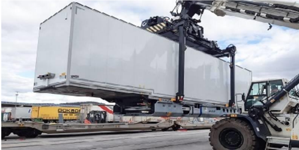
Figure 16: Example of a semi-trailer that can be handled vertically using an interface
