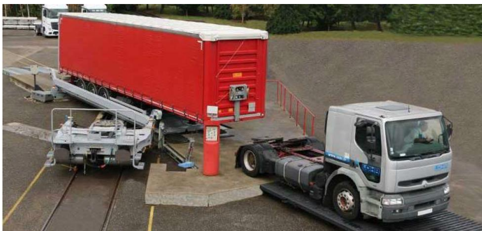
Figure 15: Example of a semi-trailer that can be handled horizontally
