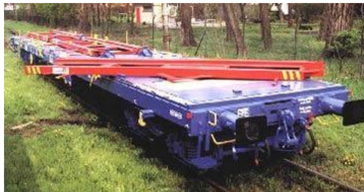
Figure 4: Example of a CT wagon suitable for the conveyance of roller units
