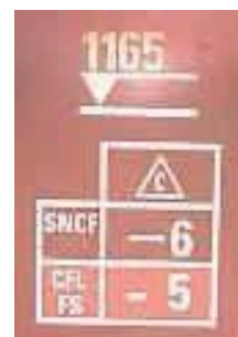
Figure 7: Marking for wagons with less favourable characteristics than those defined in IRS 50596-6, Appendices A.1 to A.4 and applicable per network
