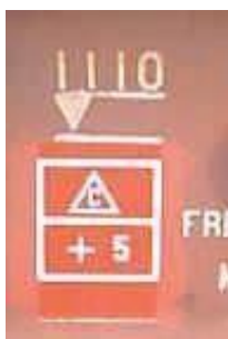
Figure 6: Marking for wagons with more favourable characteristics than those defined in IRS 50596-6, Appendices A.1 to A.4 and applicable on the entire TEN-T network
