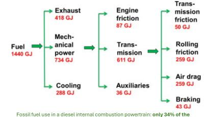
Fossil fuel use in a diesel internal combustion powertrain: **only 34% of the fuel energy is used to move the vehicle.**
