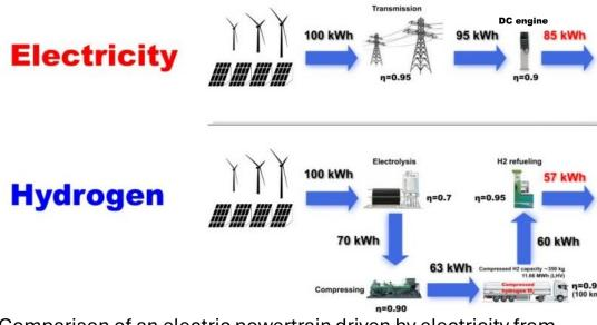
Comparison of an electric powertrain driven by electricity from the grid and a hydrogen-powered fuel-cell powertrain
