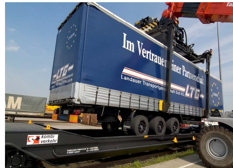
Pocket wagon for Mega-Trailers: Very low pocket platform: 270 mm above top of rail
