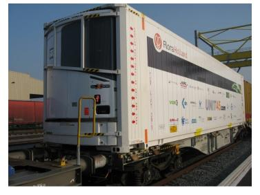
In order to satisfy the existing rules 45-foot pallet-wide swap-bodies/containers are manufactured today with patented, and hence expensive rounded corner fittings (see picture above). A modest extension of the maximum allowed semi-trailer length would enable the competitive use of every type of 45-foot intermodal loading unit in Combined Transport.
