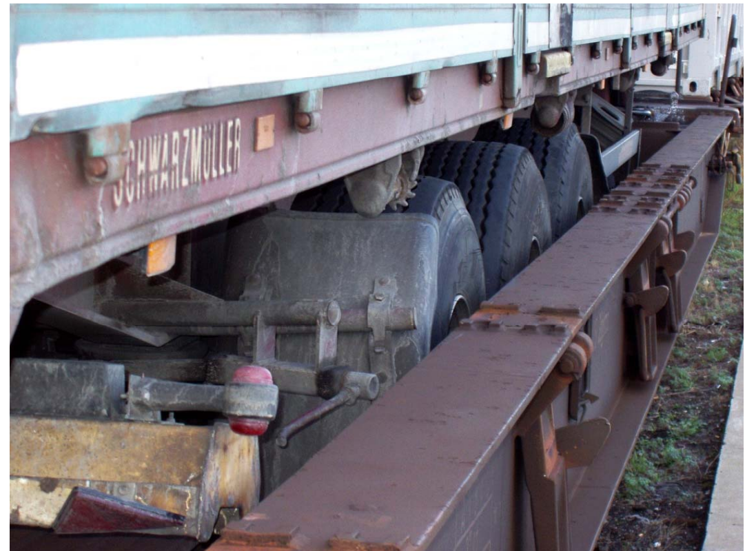
Semi-trailer loaded into a pocket wagon to minimise overall height
