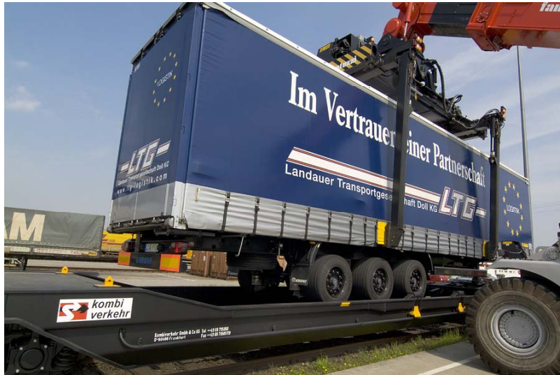
Semi-trailer loaded into a pocket wagon to minimise overall height
