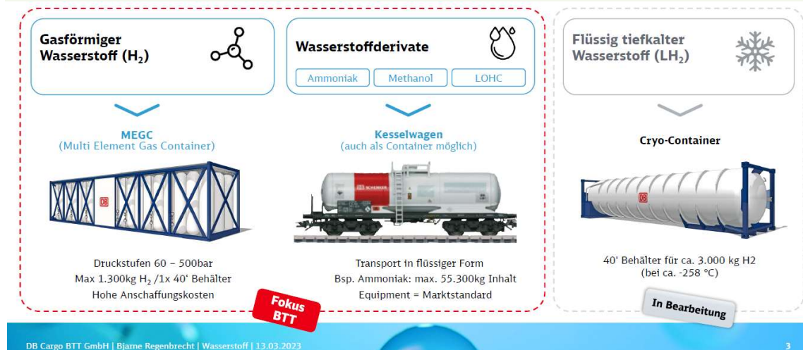
Figure 59: DB Cargo BTT's current focus for hydrogen transport covers three alternatives
