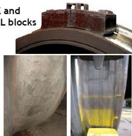
Rough wheel surface causing noise (left) vs. smooth wheel surface (right)
