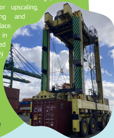
World's first hydrogen dual fuel straddle carrier
